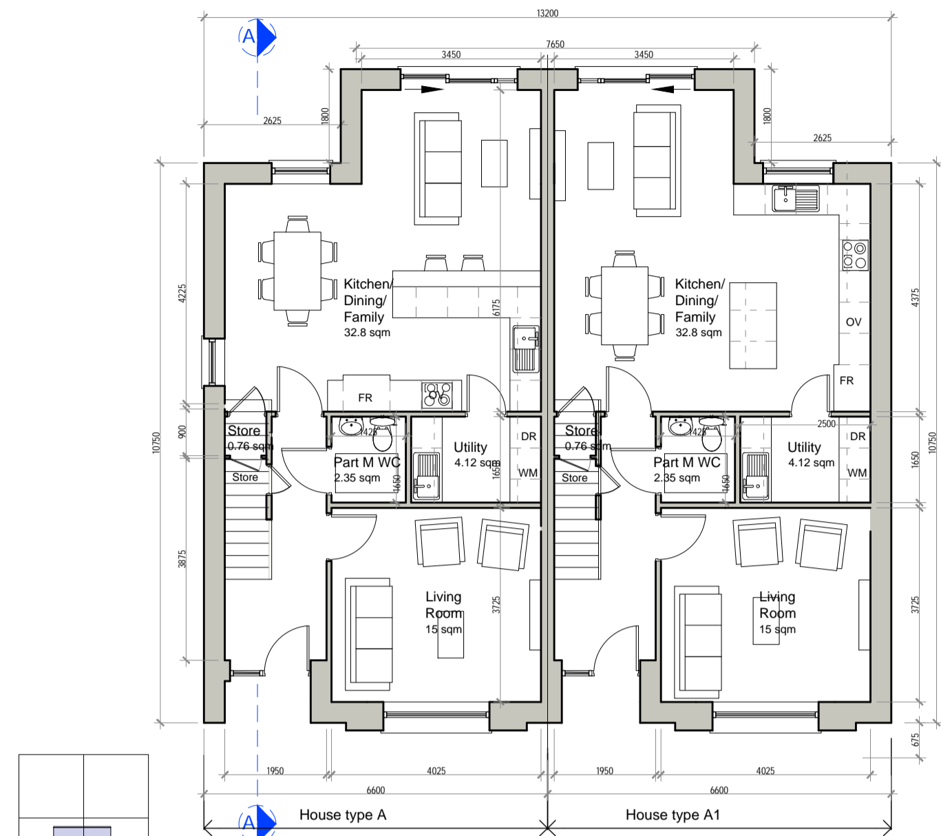
01 Type 'A' /A1 4 bed Semi D- Ground Floor Plan AREA : 65.0 sqm O/all Area : 125.4sqm / 1350 sq ft O/all Excl. stairwell to 1st floor: 123.3 sqm/ 1327sqft
